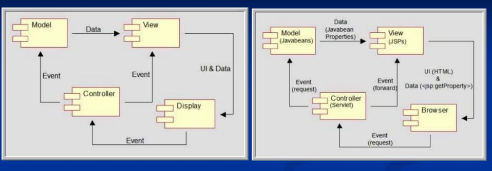
A simple interaction diagram of MVC is shown below. The Model holds all the data, the View paints UI and retrieves data to generate dynamic display, and the Controller is responsible for logical processing and delegation to Model and View.
